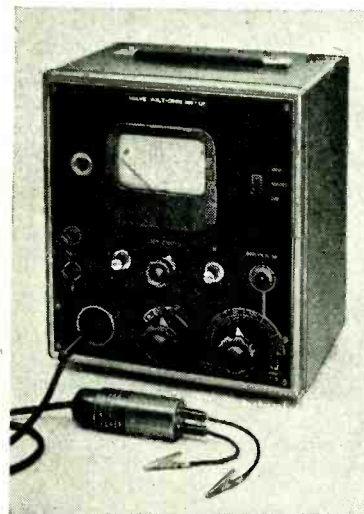
Wolf soldergun with drum of resin-coated solder fixed on the hand grip and (right) Mullard valve volt-ohm meter type E7555 with an r.f. probe.
